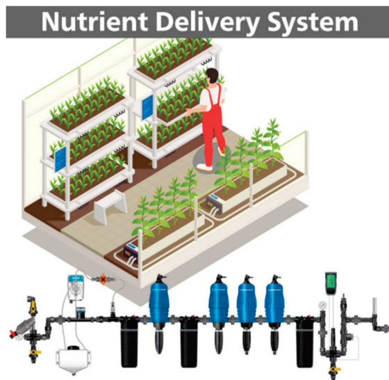
Figure 4. Nutrient delivery system of CBSO-PID and drip irrigation system.
