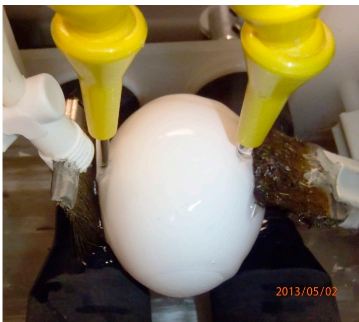
Figure 3. RF equipment to pasteurize in-shell eggs with a parallel plate array of electrodes, (a) Schematic representation [52]; (b) actual view of the system (Photo credit: USDA ARS ERRC).
