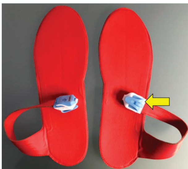
Figure 3. Example of a pair of insoles with integrated force sensors that were used for the gait analysis. The electronic hardware is located in a small box (yellow arrow) that is connected to the soles by a cable. The insoles are about 2–3 mm thick, so the soles do not significantly interfere with walking.
