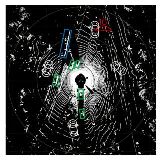
**Figure 8.** Adapting object rotation and position based on proximity and default parameters: green represents car objects, blue represents bus objects and red area indicates a horizontal range of  $\pm 10$  m within which the synthetic cars (white cars) are generated.
