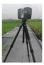
Figure 3. TLS sensor for data collection.
