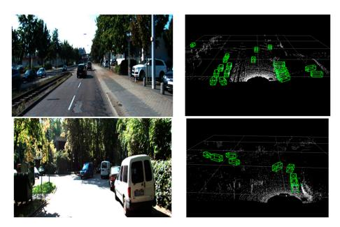
**Figure 6.** Actual detection effect diagram in KITTI dataset (left are the pictures of the real scenes, right are the detection 3D bounding boxes predicted in the point cloud).
