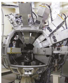
Figure 20. Diffractometer of iBIX.
