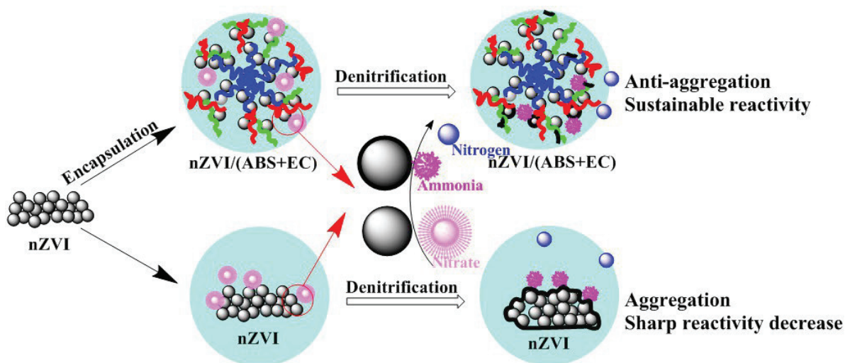
Figure 11. Denitrification mechanism of nZVI/(ABS + EC).
