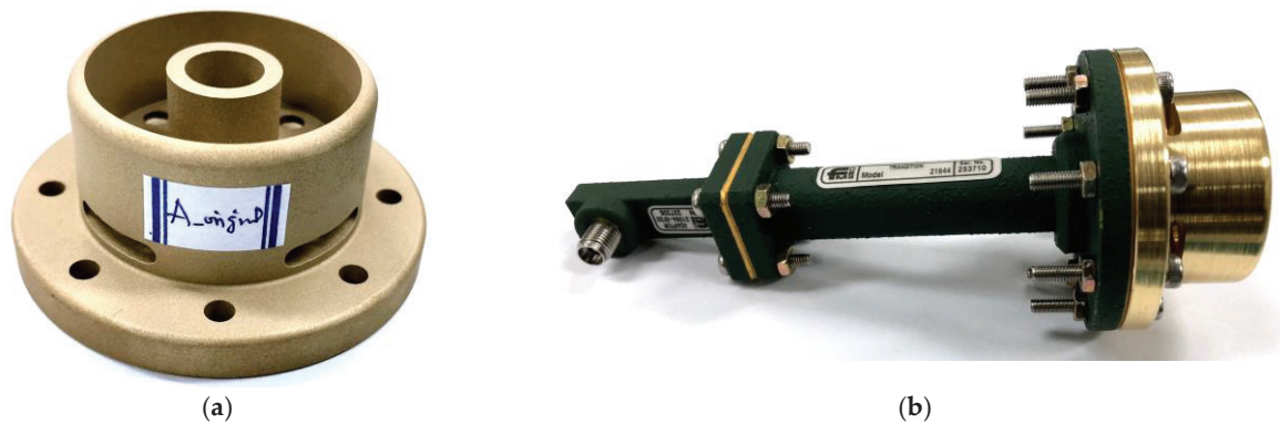
Figure 16. Photos of fabricated and assembled CRHA. (a) CRHA without EM slots. (b) CRHA with EM slots.
