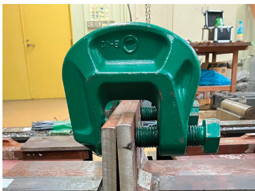
Figure 4. Vise used for the seismic retrofitting of steel structures.
