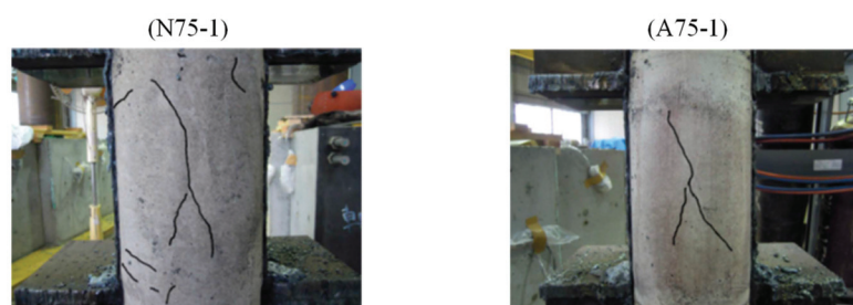
Figure 8. Cracks on inner concrete after test.
