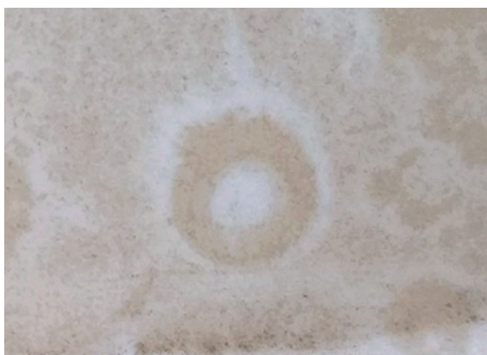
Figure 1. Dust map of surface charge distribution with a hollow ring [58].
