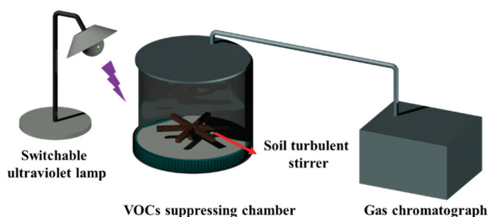
Figure 1. System for evaluating the VOC-suppressing foam.
