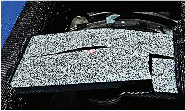
Figure 8. Brittle behavior in the carbon fiber specimen (i.e., CF_TrE25%).
