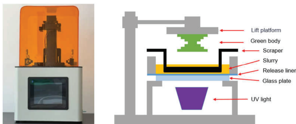
Figure 1. DLP printer and schematic diagram.
