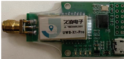
Figure 12. The UWB node. The device we use is produced by China Jiuling electronics manufacturer, whose Chinese name is printed on the surface of the device.
