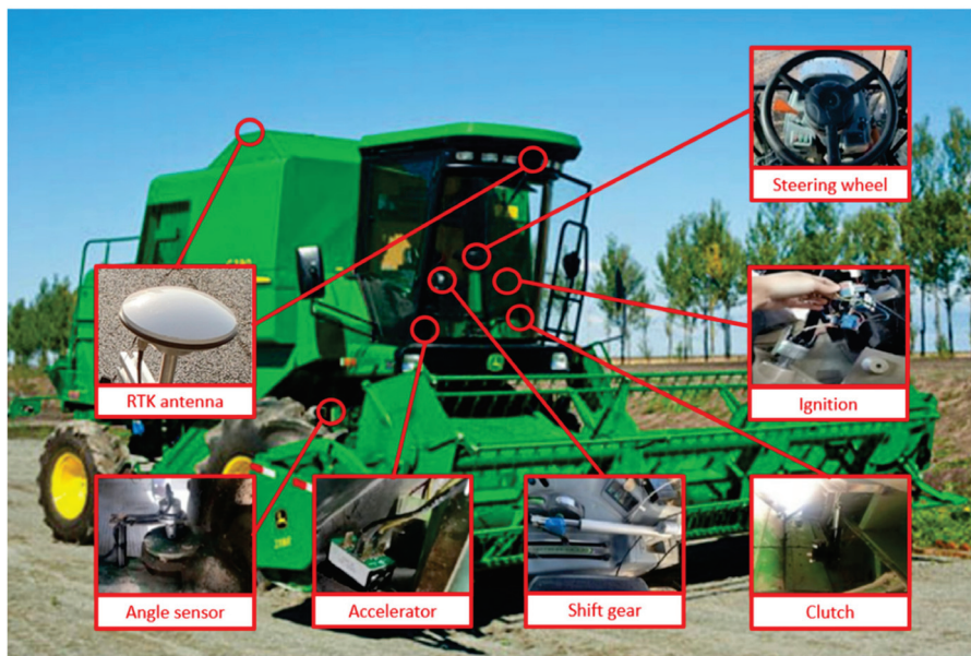
Figure 14. Reconstruction of the electric control system for the combine harvester.
