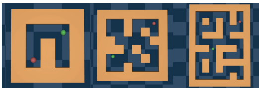
Figure 12. Umaze, Medium, and Large three maze environments, Maze2D is a navigation task. The test goal is to find the shortest path to the target point by combining the sub-optimal trajectory with the offline RL algorithm. In the illustration, the green dots represent the current position of the agent, while the red dots indicate the target points that the agent needs to reach.
