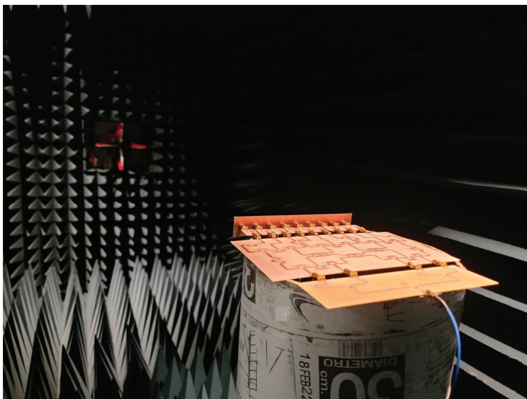
Figure 12. Prototype of the full system measured experimentally in a far field anechoic chamber.
