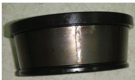
Figure 17. The fault on the inner race.
