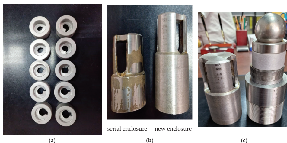
Figure 9. The newly designed valve for pilot field tests: (a)—duraluminum turbulizers; (b)—serial and new valve body; (c)—valve of new design.
