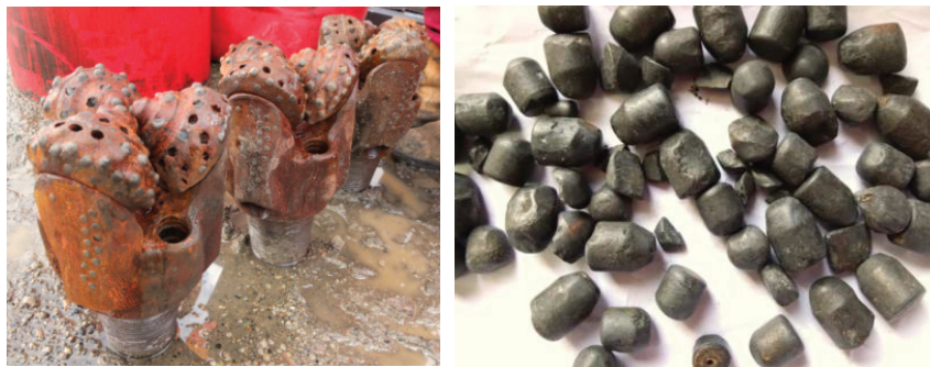
Figure 1. Tooth loss phenomenon of tri-cone drill bits in high-temperature geothermal drilling.
