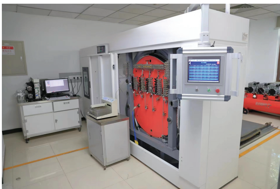
Figure 1. Large-scale physical simulation experimental equipment for MEOR.
