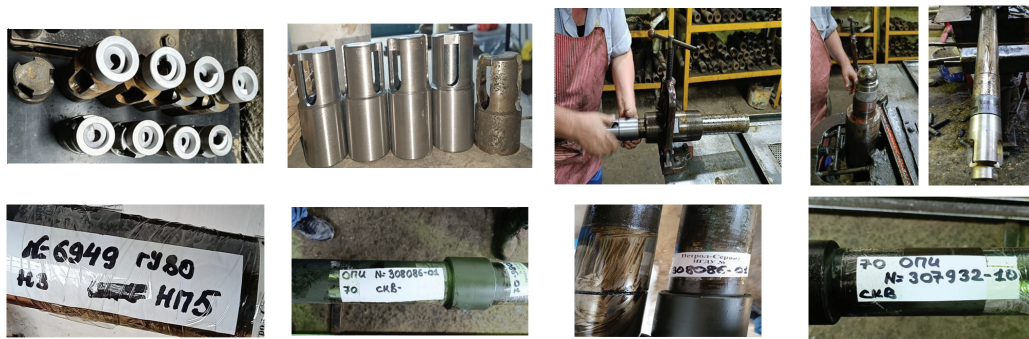
Figure 10. Installation of newly designed valves on DRP pumps.
