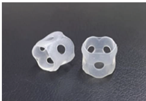
Figure 6. Silicone rubber, which is sold as a stationery item, can be used for attaching the main body of the hearing aid to the temple of the glasses or headbands.
