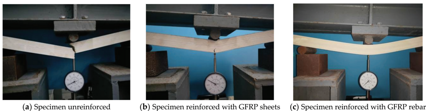
Figure 5. Failure mode of PVC-based WPC specimens.
