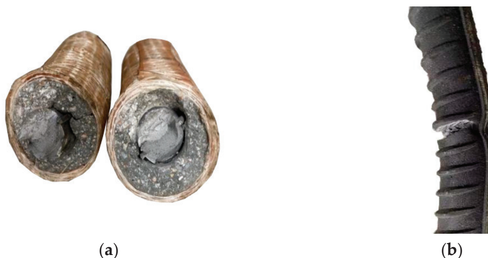
Figure 3. Fracture morphology of specimens. (a) Fracture morphology of FCCC-R specimen; (b) Fracture morphology of ordinary rebar specimen.
