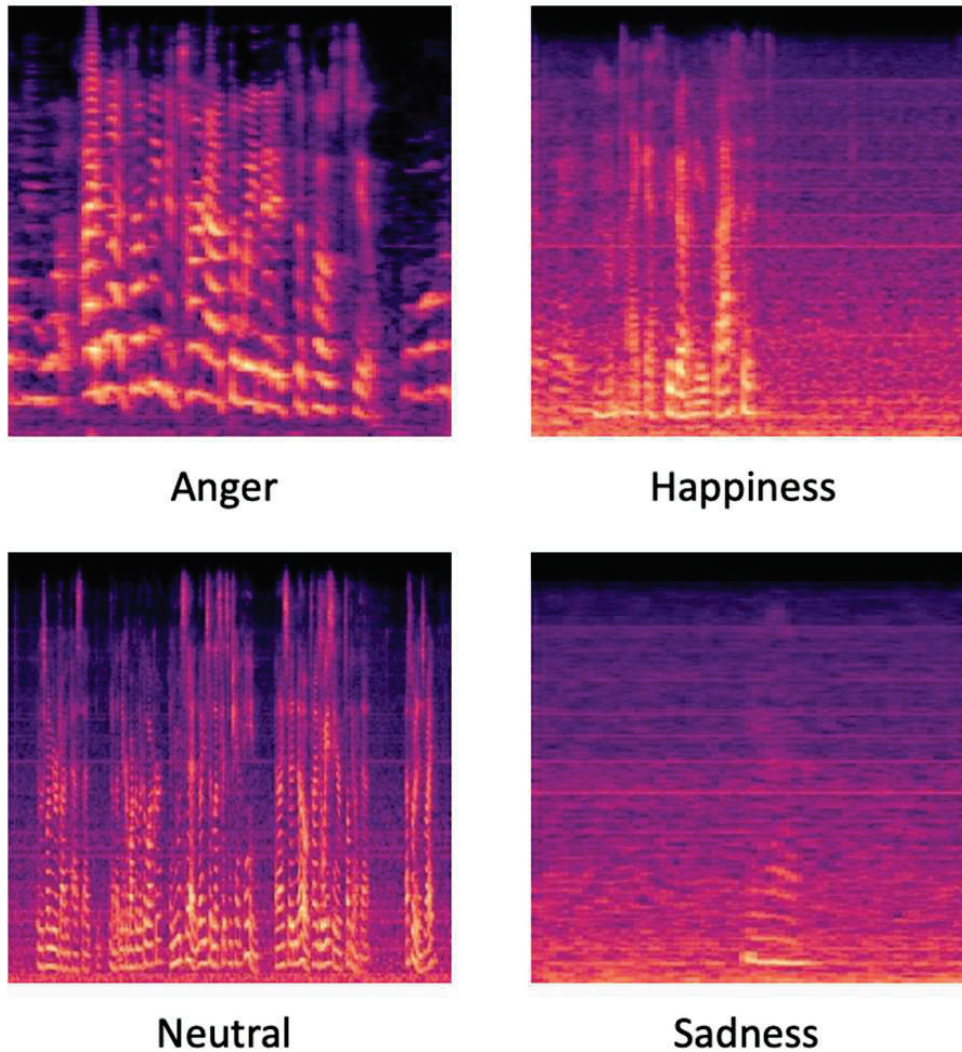
Figure 3. Differences between classes Mel spectrogram.
