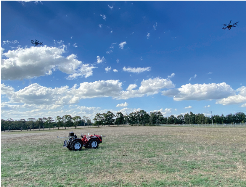
Figure 15. UAV–UGV range-based collaborative localisation experiment.
