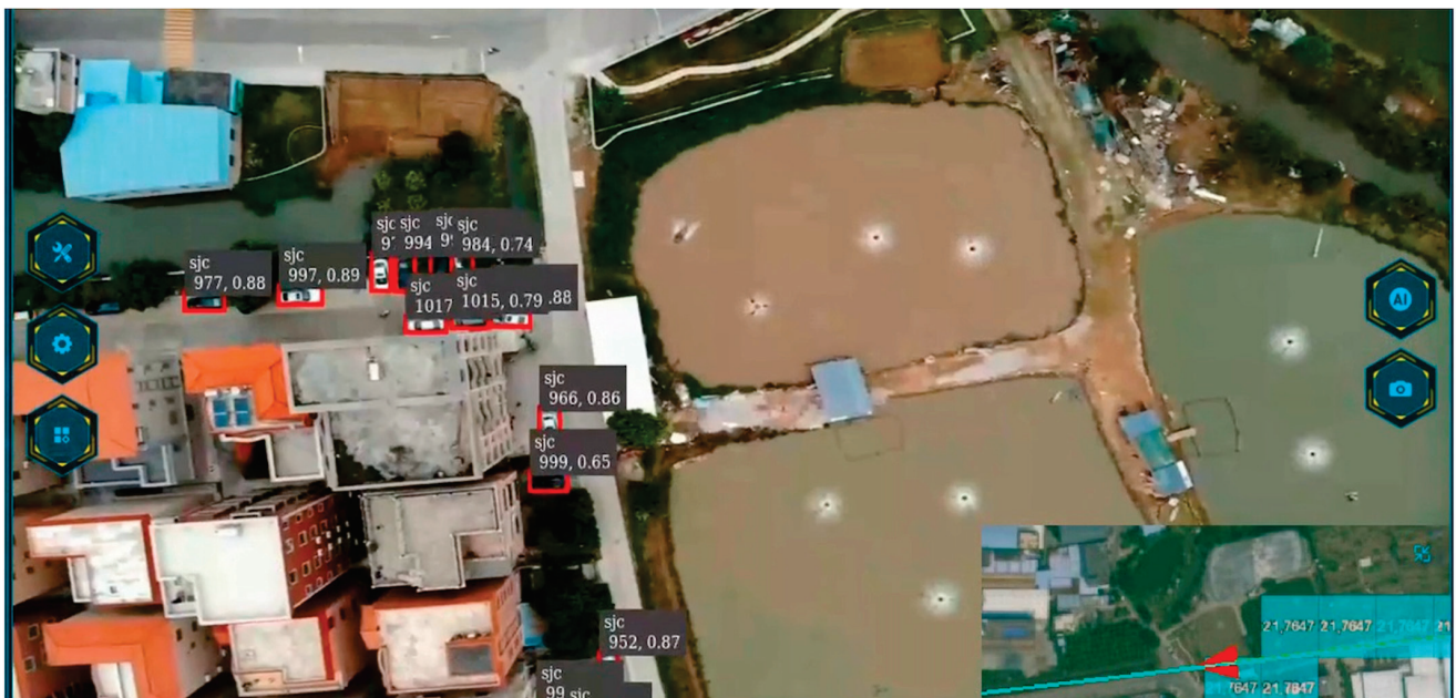
Figure 15. UAV inspection interface. It shows a scene diagram of real-time detection and tracking of high-altitude inspections, and the UAV flight route can be seen in the lower right corner.
