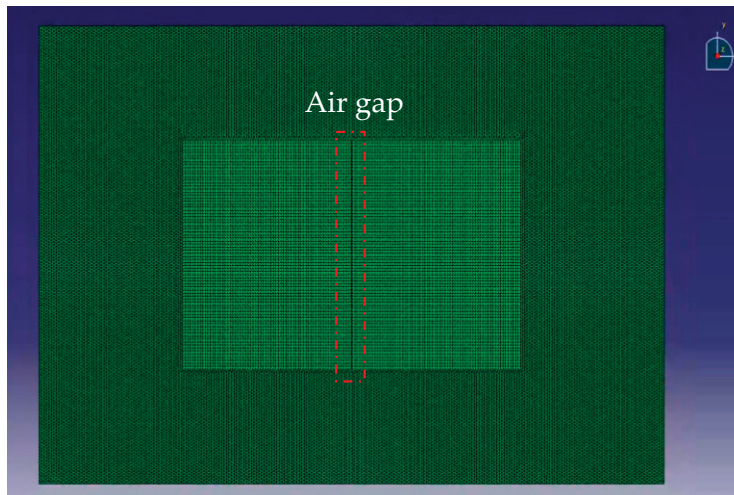
Figure 13. Finite element model of the window-wall assembly component with air gap.
