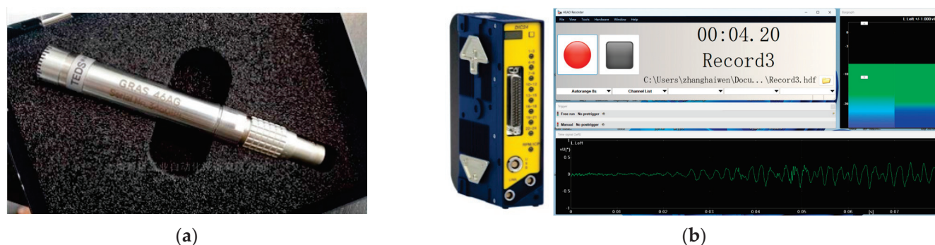
Figure 4. Test equipment: (a) GRAS sound sensor; (b) DATArec 4 DIC24 data acquisition instrument.
