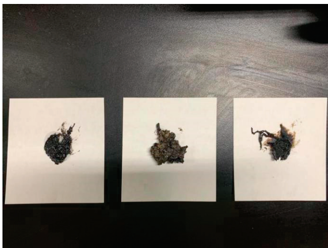
Figure 4. Sand filter pipe blockage.
