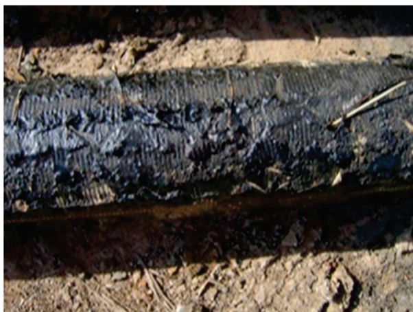
Figure 11. Crude oil agglomerates and adsorbs stainless steel wire winding screen tubes.
