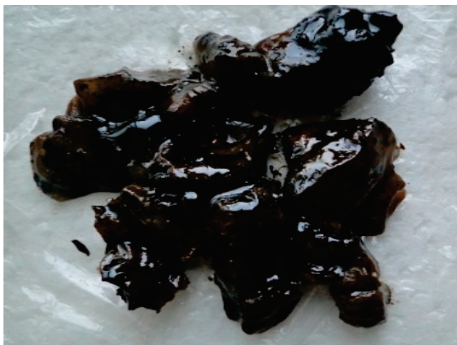
Figure 3. Oil production pipeline blockage.
