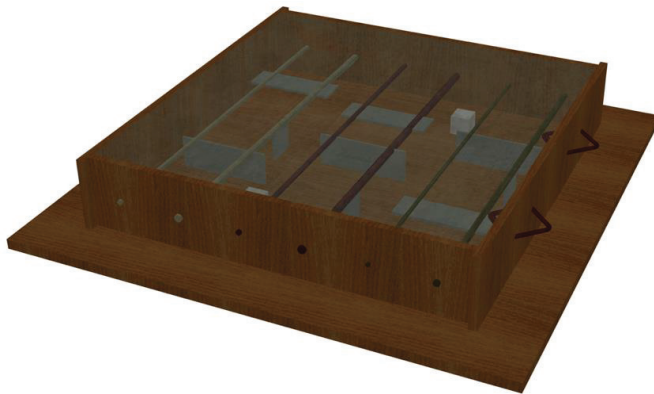
Figure 4. Three-dimensional scheme of Slab Q with simulated damage in the concrete.
