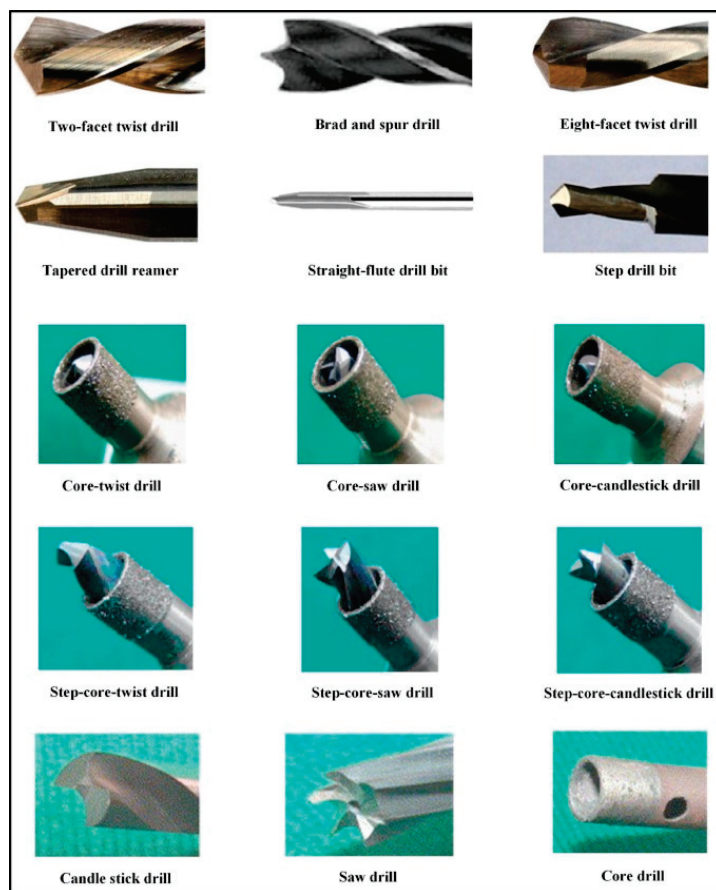
Figure 2. Various drill geometries employed in the drilling of composites [15].
