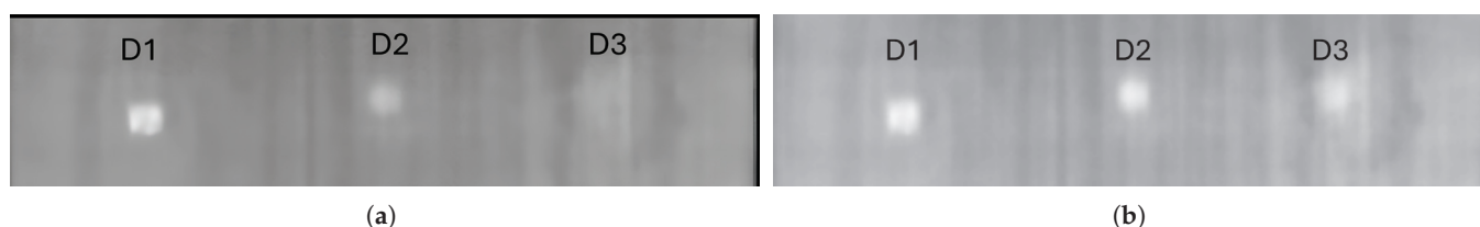
Figure 6. Comparison between images with and without processing. (a) Top section of raw data, (b) data processed with TSR.
