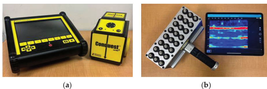
Figure 6. NDT devices used: (a) GPR device, (b) PAU device.
