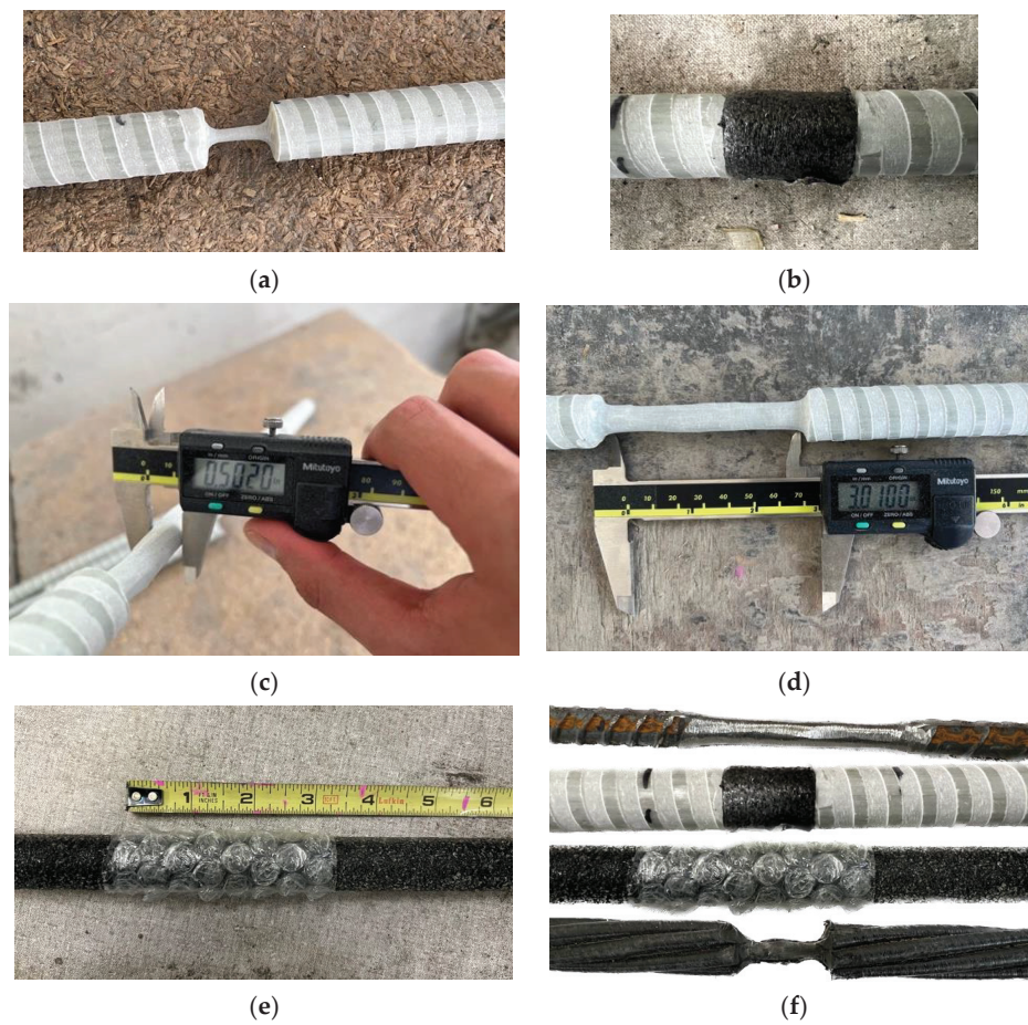
Figure 2. Damage introduced in bars. (a) Cross-section rupture, (b) covered rupture defect, (c) reduction in cross-section, (d) 3 inches of cross-section defect, (e) 3 inches of debonding defect, (f) different defects in bars.
