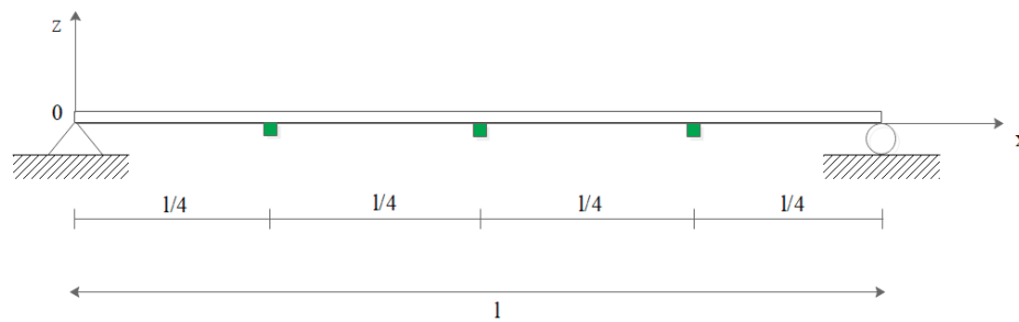
Figure 19. Simply supported beam and sensor locations.
