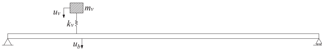
Figure 2. Lumped spring mass moving on a simply supported beam.
