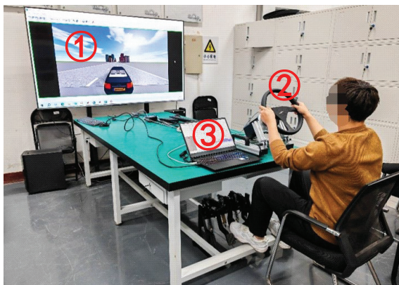
Figure 8. Driver-in-the-loop platform; ① Prescan visualization ② SensoWheel force feedback system ③ Human–machine co-driving algorithm.
