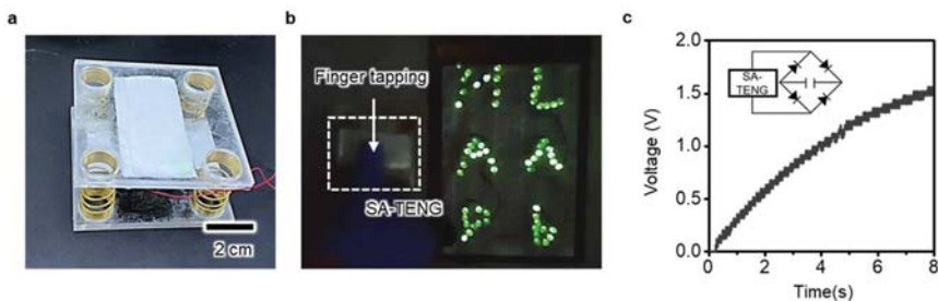
Figure 4. A fabricated SA-TENG and its demonstration of operation. The electrical output generated from the SA-TENG by a simple finger tapping motion enables simultaneous lighting up of the tens of LEDs. Applying the vertical cyclic force on the device charges the conventional capacitor.
