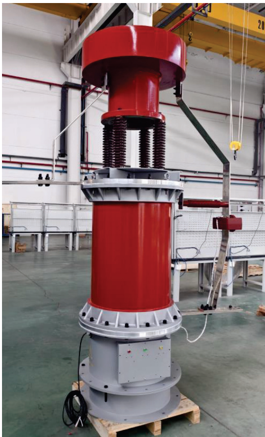
Figure 10. Overall physical image of the fault current limiter.
