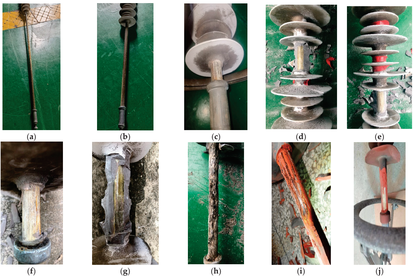
Figure 15. Aging composite insulators after dissection: (a) No. 1; (b) No. 2; (c) No. 3; (d) No. 4; (e) No. 5; (f) No. 6; (g) No. 7; (h) No. 8; (i) No. 9; (j) No. 10.
