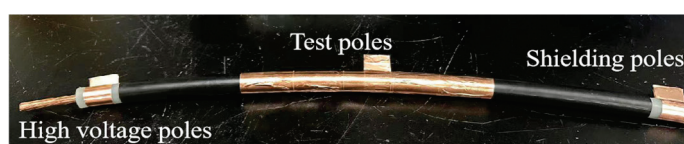
Figure 1. The cable segment sample with three electrodes used in the measurement.
