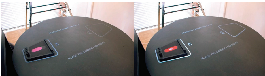
Figure 14. A moving slider is projected in support's cavity.
