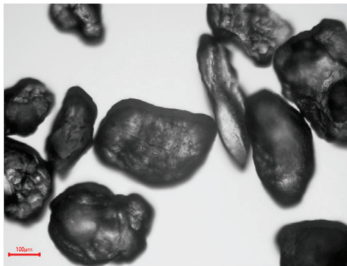
Figure 1. Micrograph of the sand particles used as projectiles impacts.
