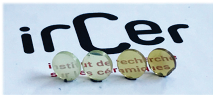
Figure 3. Transparent \text{Ho:Lu}_2\text{O}_3 ceramics with various \text{Ho}^{3+} doping rates (from the left to the right: 0.5 at.%, 1 at.%, 5 at.% and 10 at.%) sintered by SPS at 1400 °C for 15 min under 130 MPa of uniaxial pressure.
