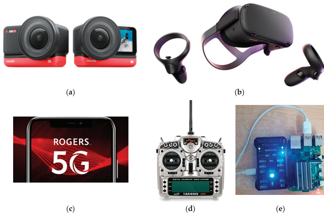
Figure 23. Connecting the VR headset (b) and radio controller (d) with an on-board 360-degree camera (a) and Raspberry PI (e) to obtain the flight data and display them on the VR screen in real time using the 4G/5G network (c).
