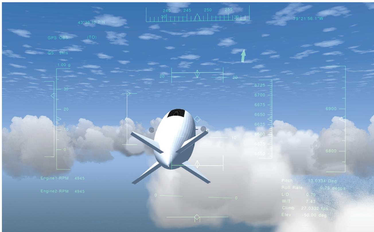
Figure 5. HUD elements were presented on the screen of the FGFS to increase pilots' situational awareness.
