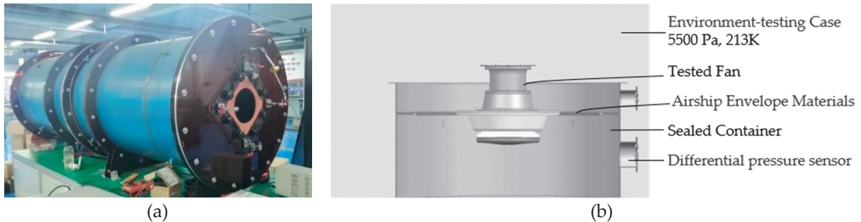
Figure 10. (a) Fan performance test bench for the ground condition; (b) Fan performance test bench for stratospheric condition.
