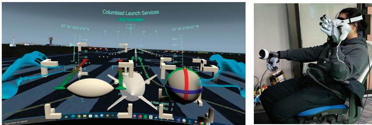
Figure 24. View from within the Oculus Quest VR running the flight simulator and the actual pilot wearing the SenseGlove Nova set for command and control.
