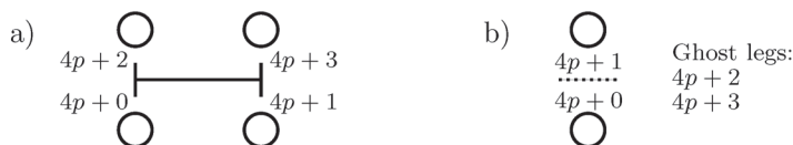
Figure 15. Assignment of leg numbers to operator legs for an operator at propagation step p . (a) Illustration of a two-site operator with four real vertex legs. (b) Illustration of a single-site operator with only two real vertex legs and two ghost legs.
