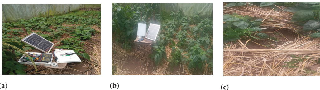
Figure 11. Visual depiction of IoT sensor setup; (a) sensors, battery and solar; (b) sensor assembled; (c) sensor deployed in cropland.
