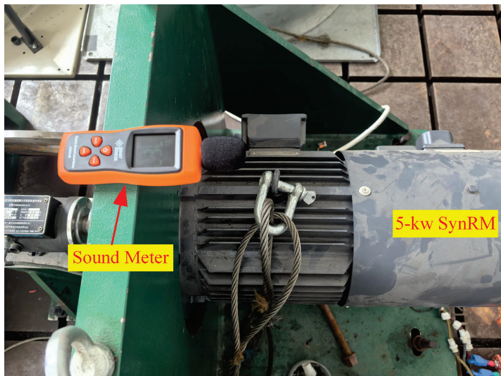
Figure 22. Collecting the noise level generated by the motor using Smart Sensor AS804B.
