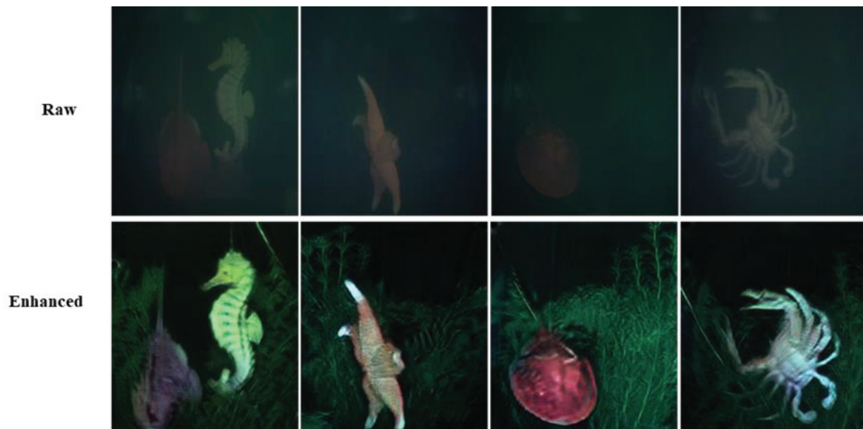
Figure 7. Comparison of images captured by the MLIS and enhanced with the optimized algorithm with the average UCIQE improved from 0.428 to 0.925.
