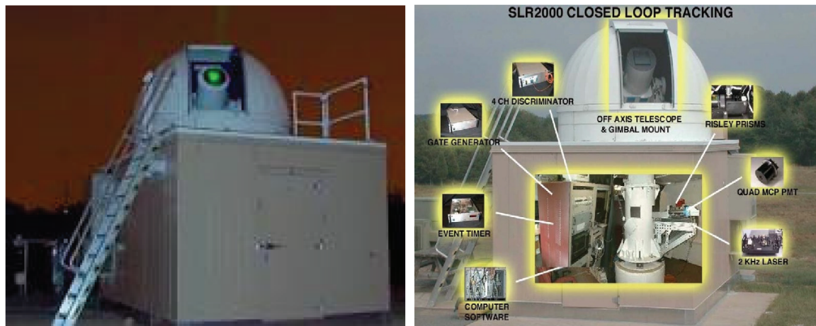
Figure 1. The prototype NASA SLR2000 system projected a 2 kHz train of low energy, 532 nm, sub-nanosecond pulses via an unobscured 30 cm primary lens in order to concentrate more photons on the satellite while simultaneously eliminating potential eye hazards.
