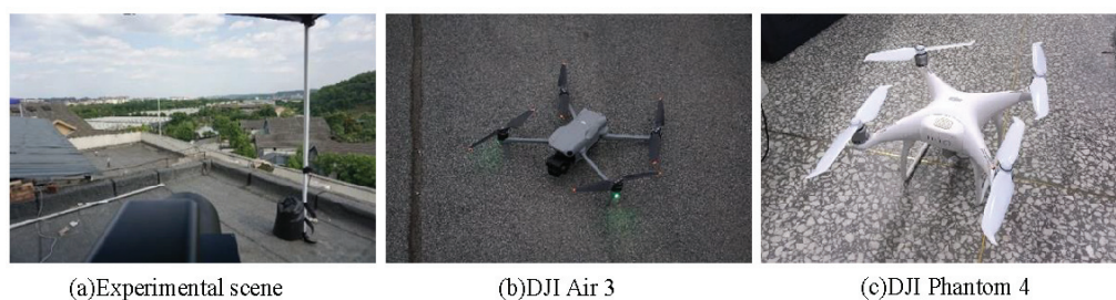
Figure 3. (a) Experimental scene, (b) the DJI Air 3 UAV with a length of 258.8 mm, a width of 326 mm, and a height of 105.8 mm; (c) the DJI Phantom 4 UAV with a length of 430 mm, a width of 430 mm, and a height of 370 mm.
