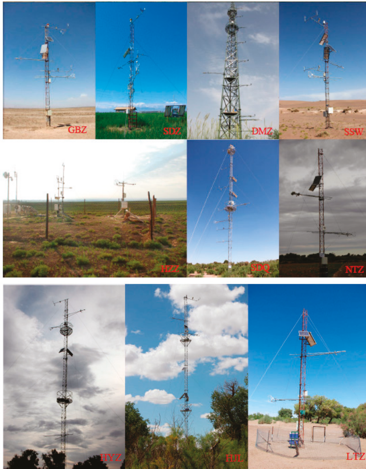
Figure 3. Photos of the 18 Heihe Watershed Allied Telemetry Experimental Research (HiWATER) stations. The two pyrgeometers that were used to record the longwave radiation were deployed at an average height of 6 m, with one facing upwards and the other facing downwards.
