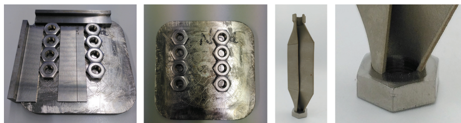
Figure 4. Hybrid manufacturing of modules on nuts with an exemplary empty module (three-quarter cut).
