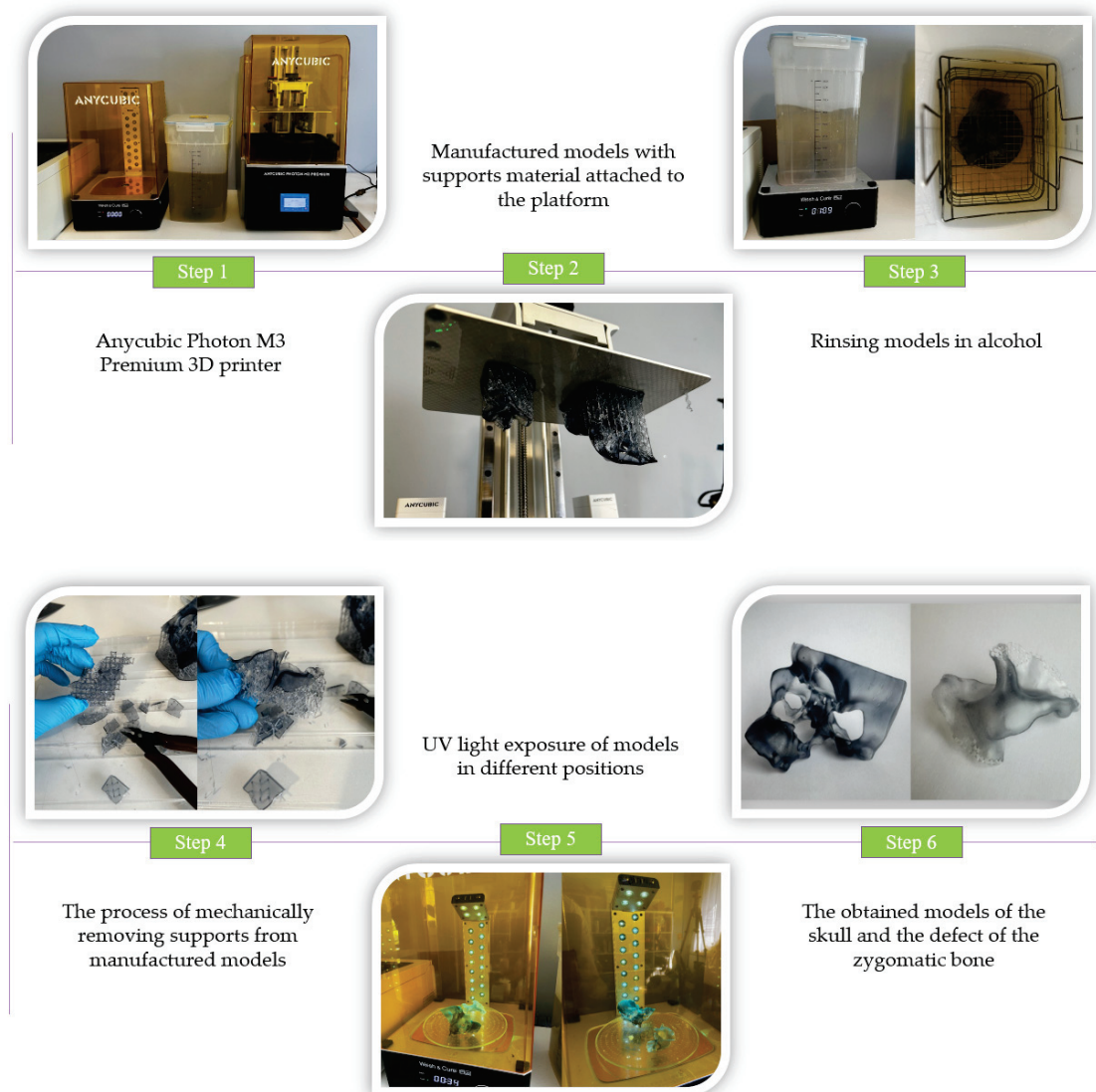
Figure 4. The process of manufacturing models using the example of the first patient.
