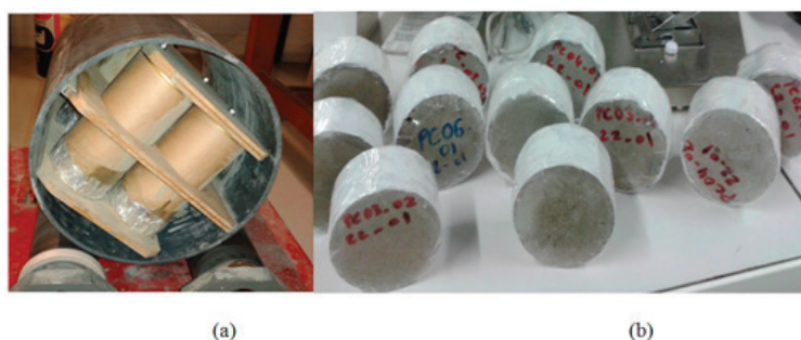
Figure 1. A device used during the cement paste's hardening (a), specimens used for the study (b).
