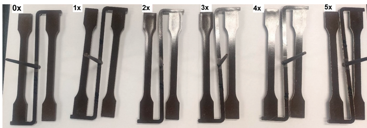
Figure 2. Samples from the original composite (0x) and subsequent reprocessing cycles (1x–5x).
