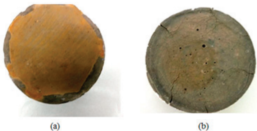
Figure 11. Observed damage of samples after two months of exposure to sulfate solution: (a) early-age exposure, (b) matured cement pastes.
