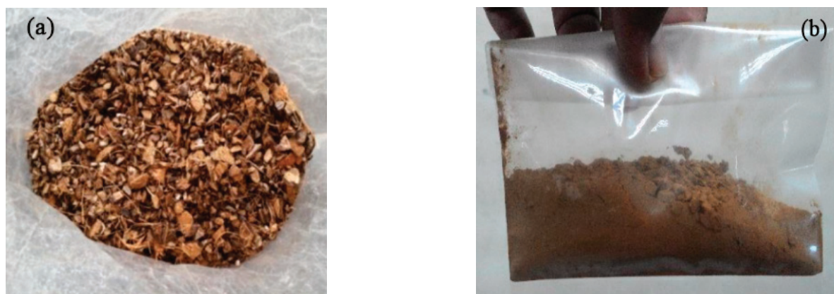
Figure 3. Preparation of coconut shell: (a) chips (20 mm) and (b) fine powder.
