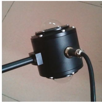
Figure 3. Developed spectral albedometer for one band.
