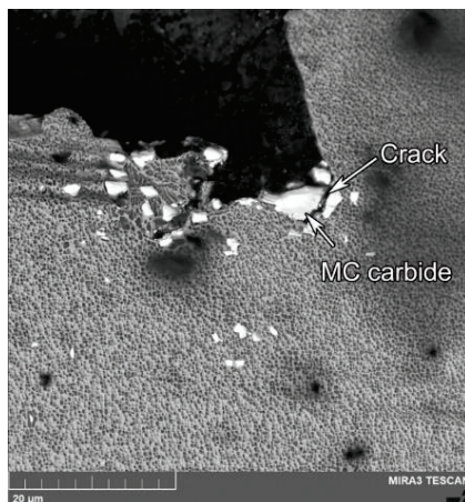
Figure 7. MC carbide near the fracture surface after tensile test at 650 °C.
