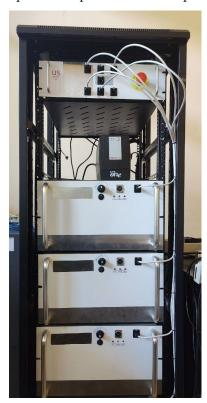
Figure 4. Parallel CLLC resonant converter system physical configuration.
