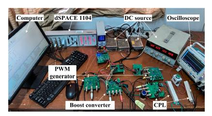
Figure 10. Experiment platform of boost converter with CPL.
