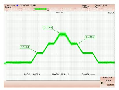
**Figure 8.** Positive variation of total current through the DC bus. Frequency is not detected in DC mode and its value appears as stars. Time scale: 10 A/div.
