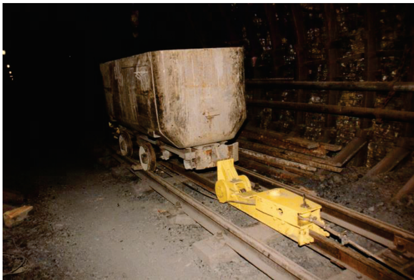
Figure 1. Transport system with a rope winch in an inclined underground tunnel.
