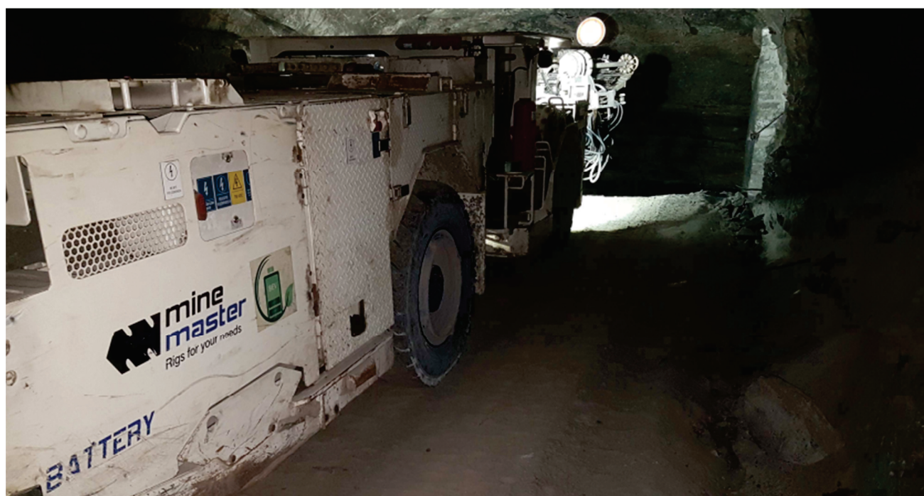
Figure 9. Photo from braking effectiveness tests on a slope of 12°.
