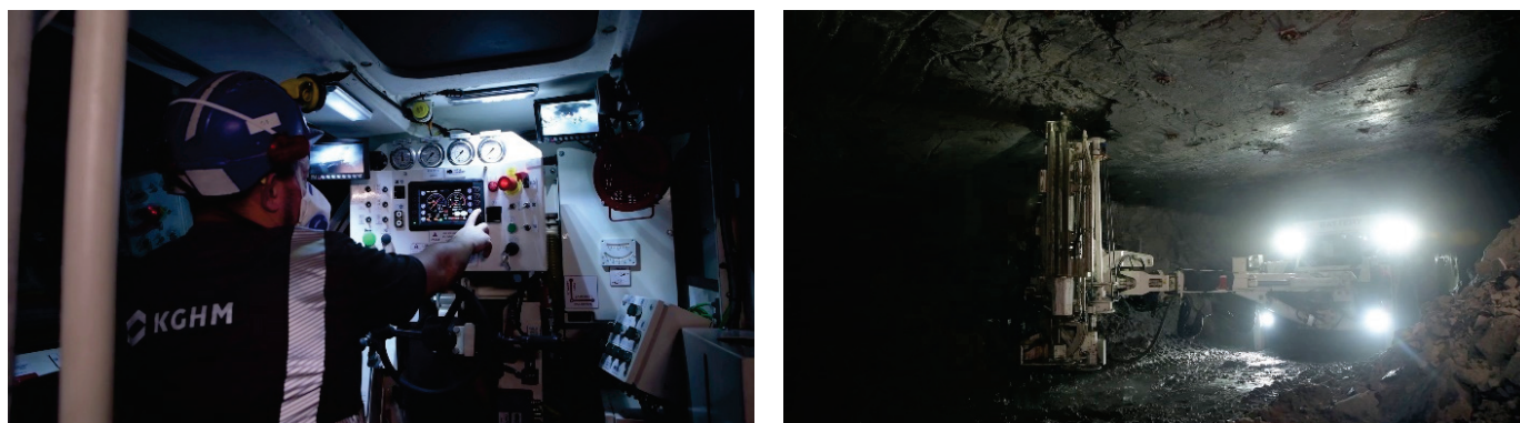
Figure 3. Photos of the Roof Master 1.8 KE roof bolter taken during the tests.
