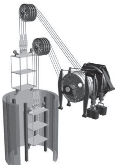
Figure 2. Hoist model with the rope winch [13].
