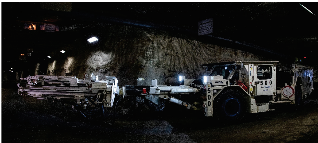
Figure 1. Battery-powered self-propelled Roof Master 1.8 KE roof bolter in the KGHM mine.
