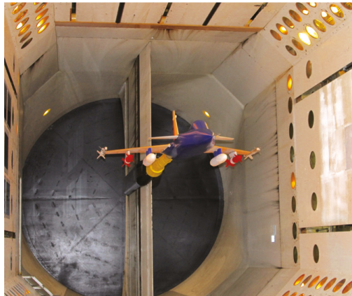
Figure 11. The generic fighter aeroelastic wind-tunnel model installed in the Transonic Dynamics Tunnel (TDT).
