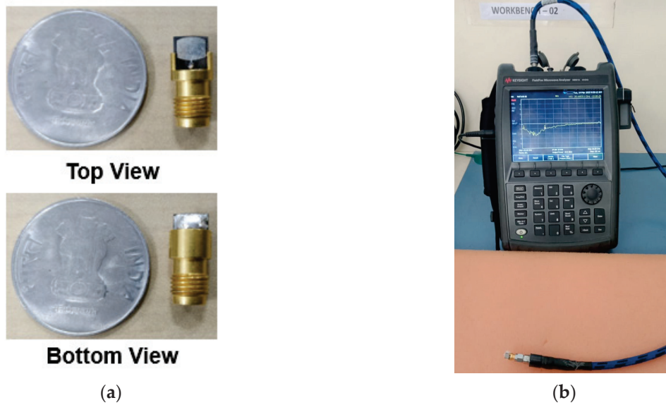
Figure 10. Photos of the antenna and the reflection coefficient measurements. (a) Photos of the antenna and (b) the measurement setup of the |S_{11}| parameter.
