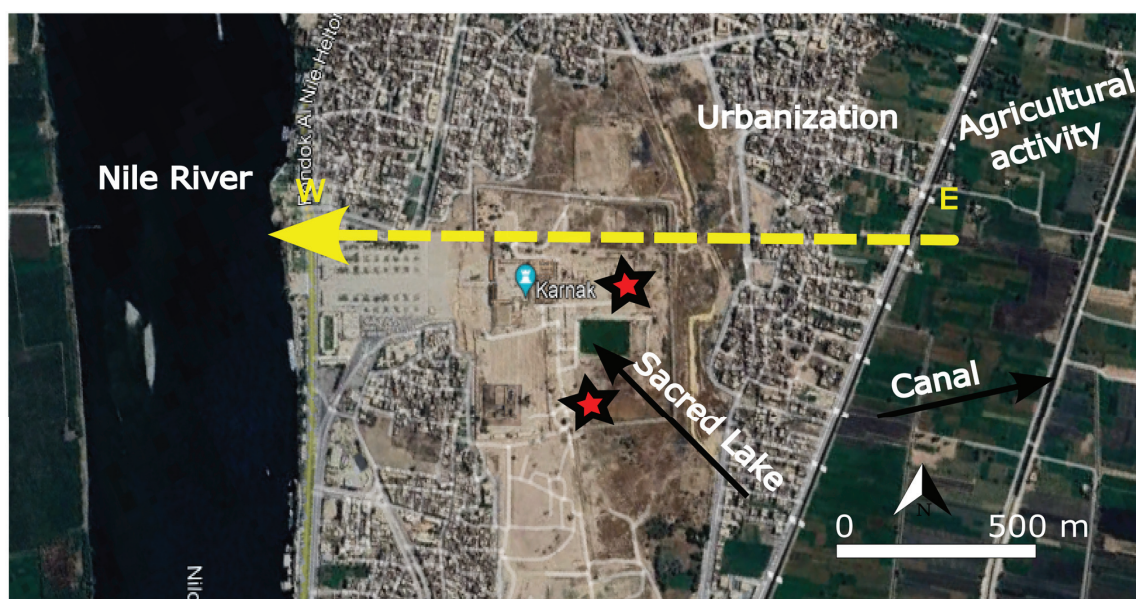
Figure 4. Various contaminated water sources in and around the Temples of Karnak. The yellow arrows indicate the flow direction of water from east to west, originating from canals, drains, cultivated lands, and houses. Salt-contaminated aquifers beneath the Temples of Karnak are marked with stars [53].
