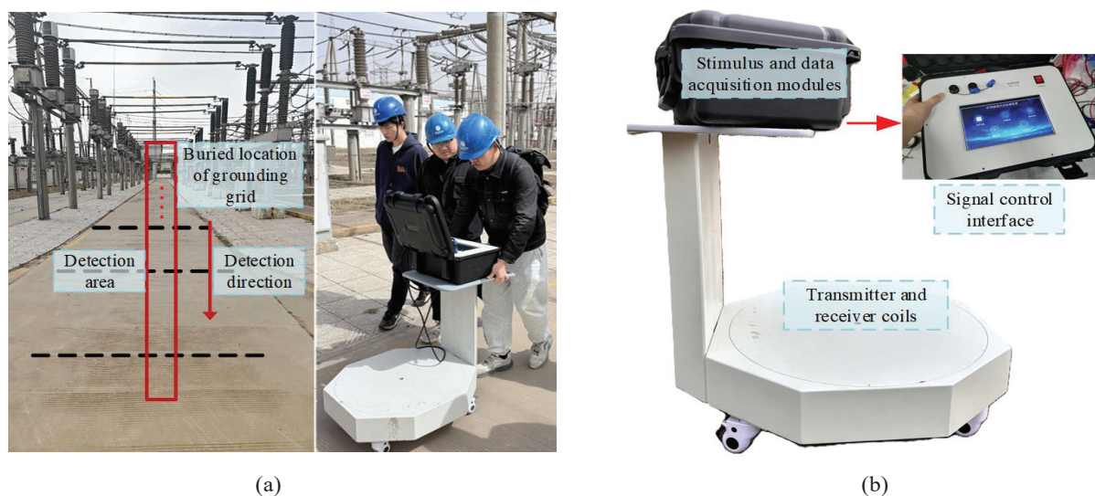
Figure 9. Field signal acquisition and detection device. (a) On-site detection schematic diagram. (b) Grounding detection device.
