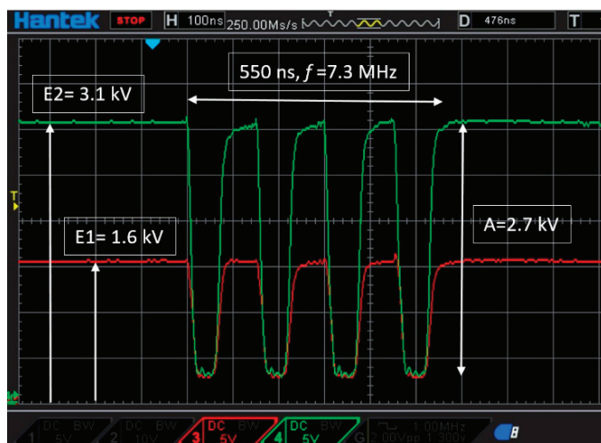
Figure 14. Voltage waveforms on drains of two STP4N150 transistors in the new generator (experiment). Scales are 500 V/div and 100 ns/div. HV probes are 1:100. Red: the waveform for the drain of STP4N150 at the T1 site. Green: the waveform for the drain of STP4N150 at the T2 site.
