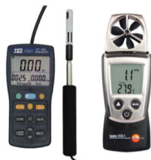
Figure 2. Test instruments: hot-wire anemometer and impeller anemometer.
