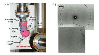
**Figure 5.** NC measurement for the T-state deoxyHbA crystal. (**a**) Experimental setup; (**b**) Typical neutron diffraction pattern of the deoxyHbA crystal. The dashed circle represents the resolution at 2.0 Å. The picture below is a close up view.
