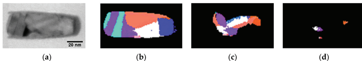
Figure 5. Cross section of a copper nano connector, (a) bright-field image, (b) first indexation, (c) second run, (d) third run. The grain highlighted in white extends as a non-dominant component after successive subtractions of the dominant grain reflections. The scan size is 110 \times 60 pixels.
