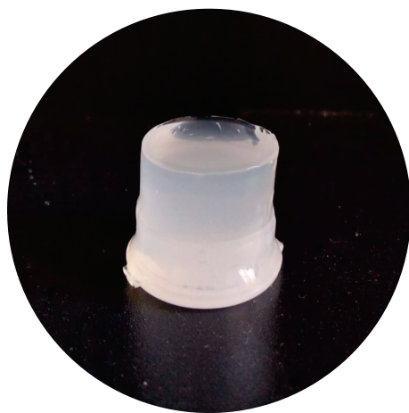
Figure 3. A \beta -chitin hydrogel camera picture. The hydrogel cylinder has a diameter of about 1 cm.
