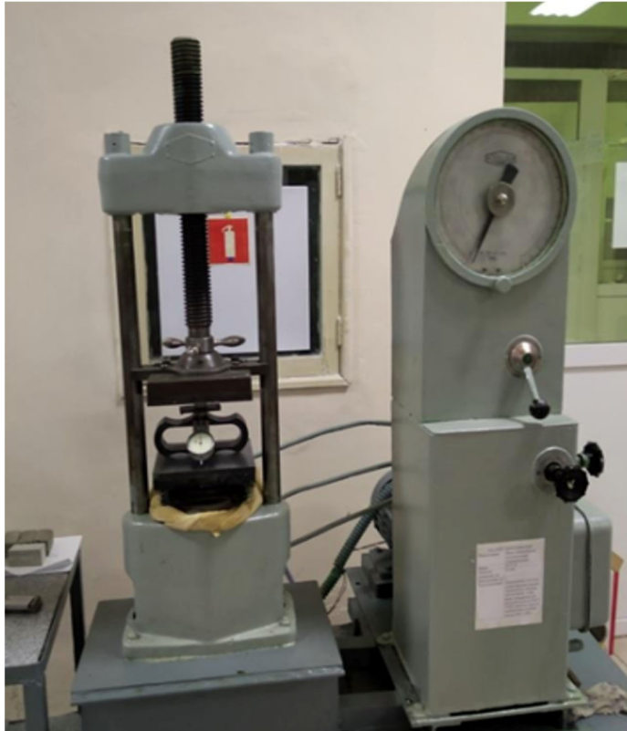
Figure 11. Compression testing of core samples using the DOSM-3-3 device.
