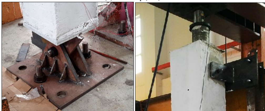
(c) Hinge supports at the joint.
