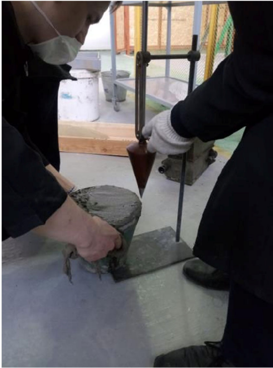
Figure 2. Workability test of the fresh concrete mixture.
