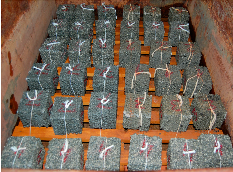
Figure 1. Test specimens in a bath in a refrigeration chamber before soaking.
