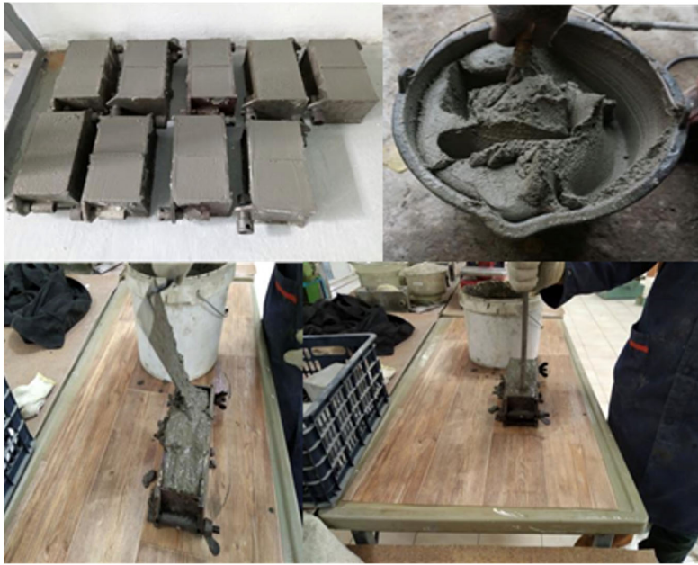
Figure 4. Sampling and preparation of control specimens.
